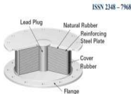
Figure 2c-Shows the base isolation with lead Rubber
