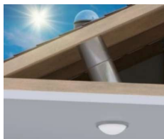
Figure 7 : Image depicts Solatubes working mechanism
