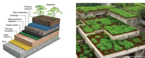
Figure 6 : Green roof with its working details
